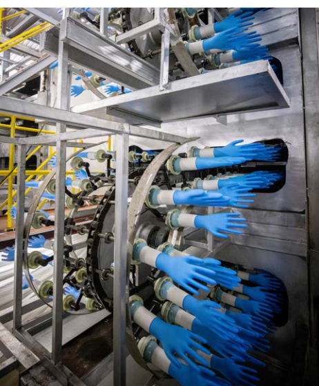
Mah Sing Healthcare's 12 automated production lines have the ability to produce 3.68 billion pieces of gloves a year.
